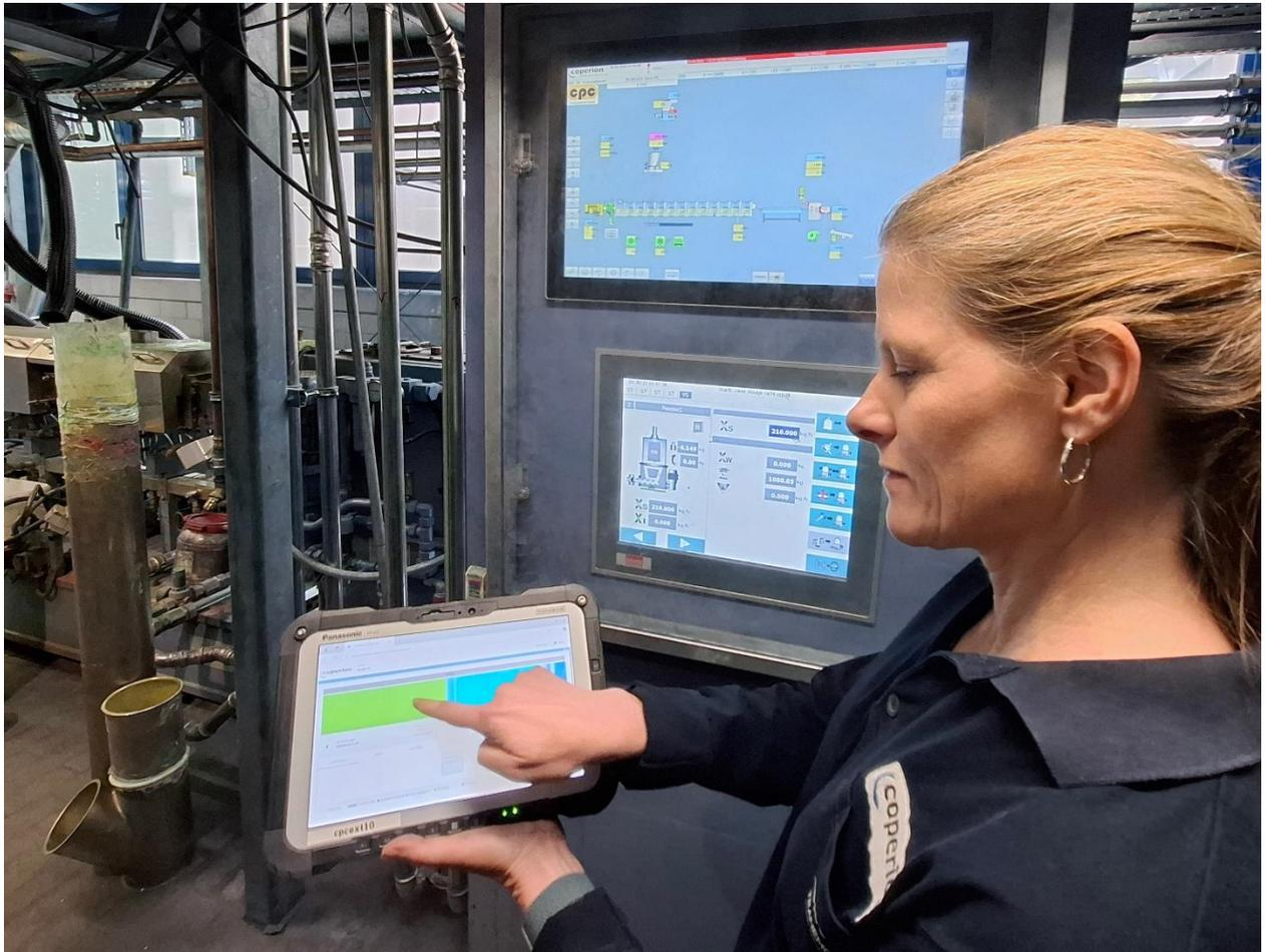
The C-BEYOND digital service platform is an important component of cpc's production planning. At any time, ZSK extruder operating personnel can enter data on the production status to the system.
