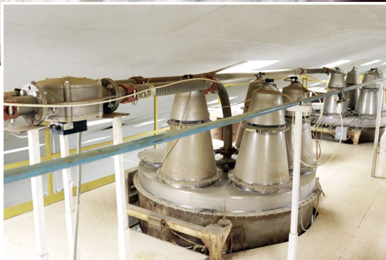
Figure 3. Coperion WZK two-way diverter valve directs material to one of two hoppers equipped with Coperion K-Tron modular cartridge bin vents.
