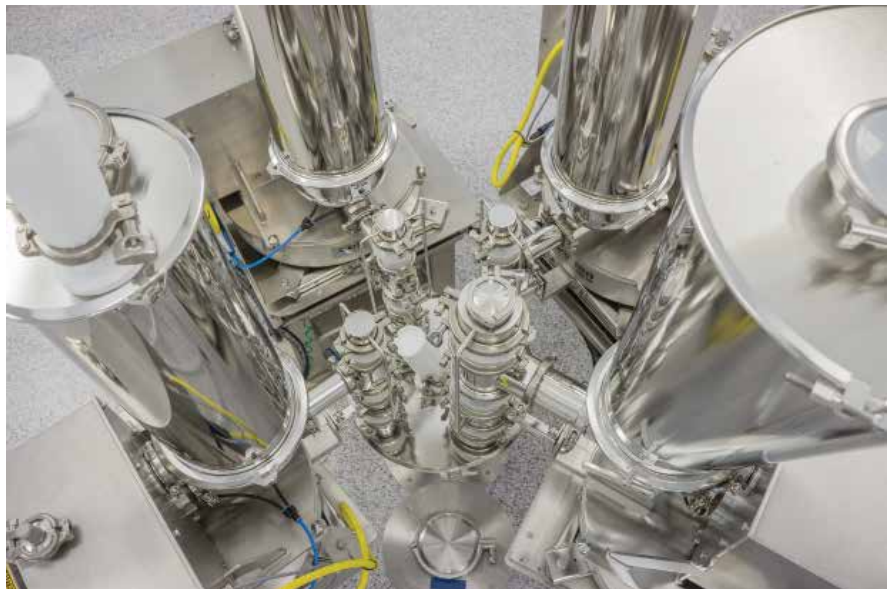
Photo 2: Multiple upper-level gravimetric feeders discharge ingredients continuously into a blender on the level below. The feeders are mounted on specialized pivoting tracks to optimize accessibility.
