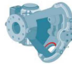
Figure 10 – One-channel diverter valve WRK with product layer.
