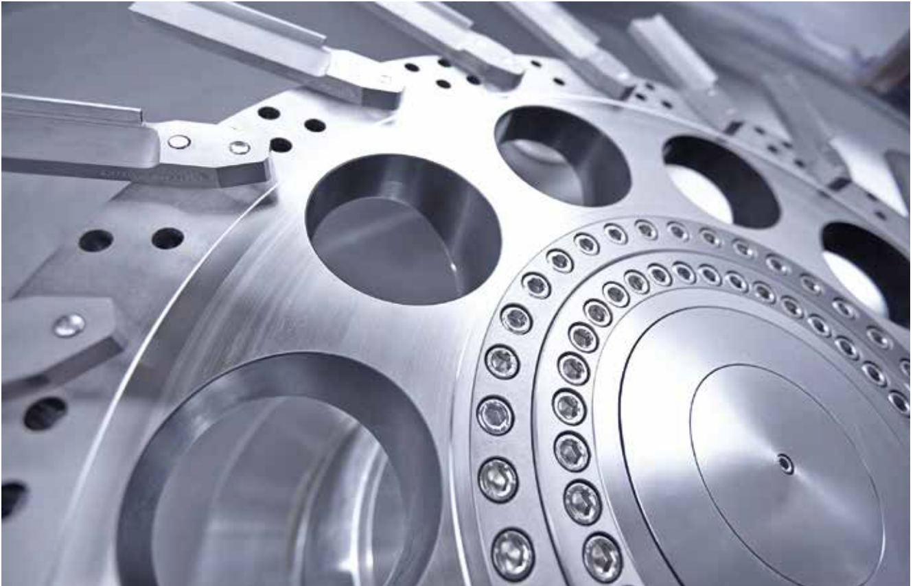
Underwater pelletization: Abrasion and corrosion combine where cutting blades come into contact with the die plate. A new wear protection alloy significantly reduces the effects of both mechanisms (© Coperion)
