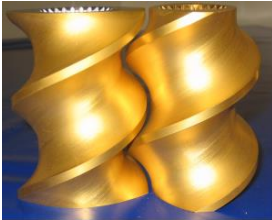
Fig.2: TiN layered screw elements for manufacturing of Polycarbonate.
