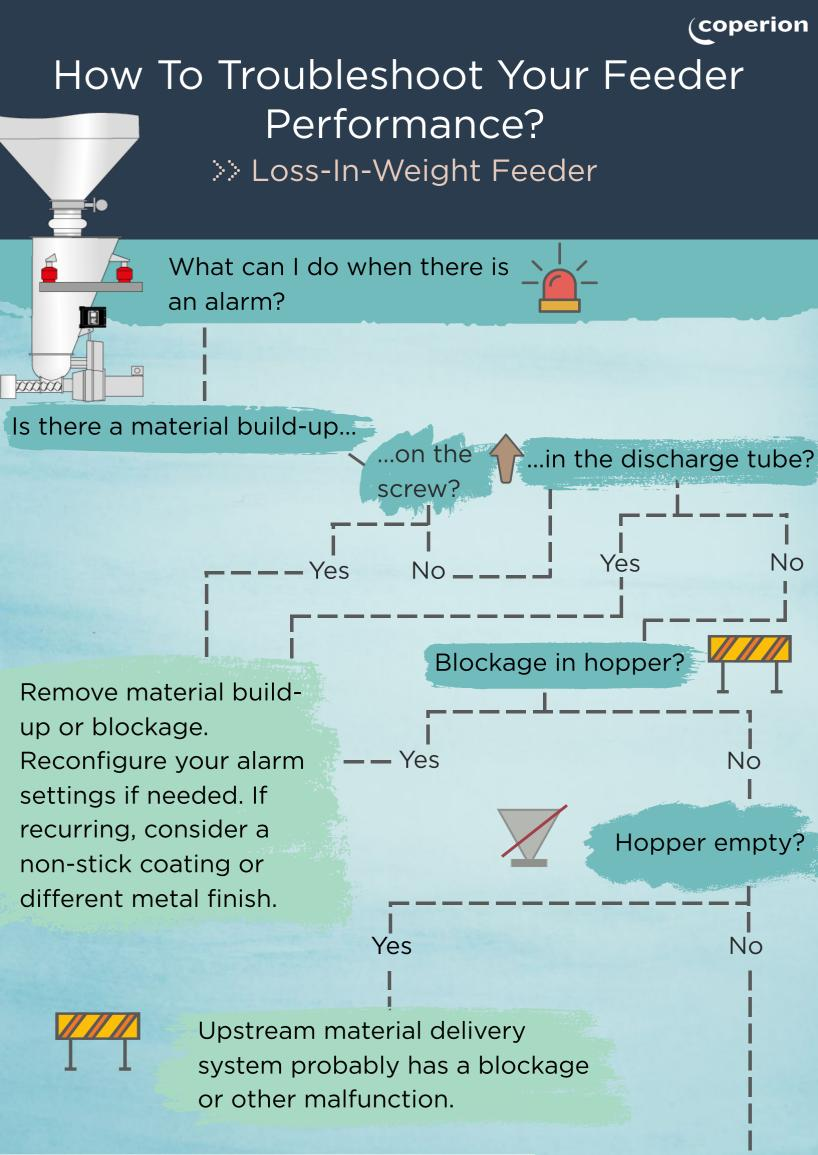
Install the feeder in such a way that the weight sensing device is shielded from the effects of environmental vibrations. Do this by ensuring that the feeder mounting is stable, using flexible connections and shock mounts, and by eliminating strong air currents near the feeder. Were the feeder's flexible connections refitted improperly during maintenance?
